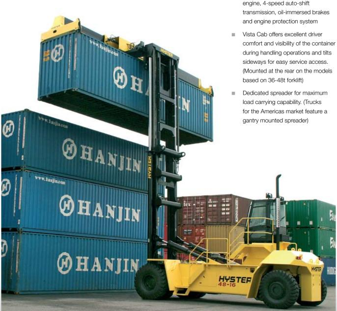
First Row Container Stackers, for stacking laden containers 3, 4 & 5 high are able to perform container shunting operations at exceptional speeds. These trucks have been purposely developed to deliver these high 'box-rates' in order to offer an alternative cost-effective solution to customers, when 2nd / 3rd row storage is not required.
